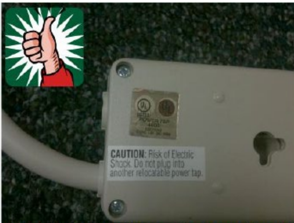
UL Listed sticker on the back of a power strip; all power strips, multi-outlet adapters, extension cords and UPSs must be UL Listed.
