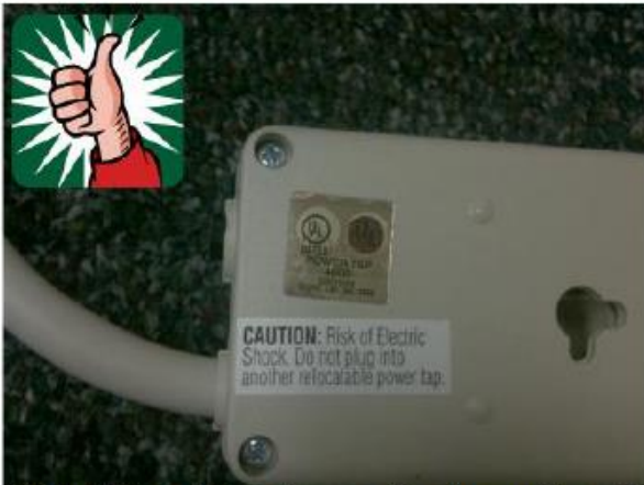
UL Listed sticker on the back of a power strip; all power strips, multi-outlet adapters, extension cords and UPSs must be UL Listed.
