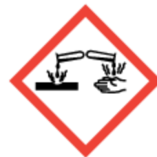
Corrosion Corrosive, skin damage, eye damage
